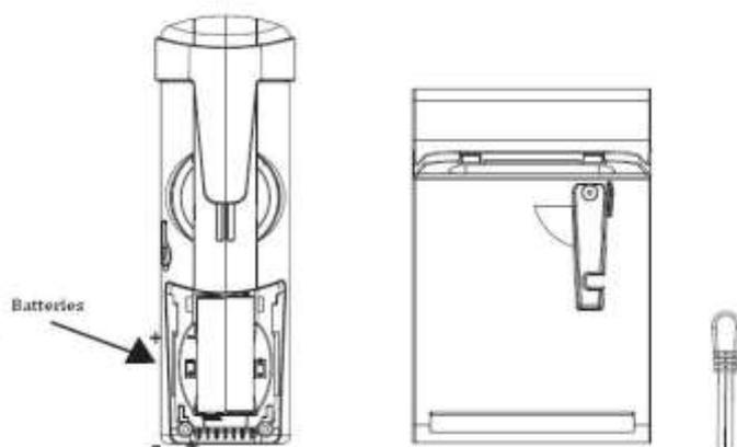
Insert the batteries into the handset battery compartment.
